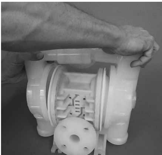
Step 10. Figure 10 After clamp bands are removed, pull liquid chambers apart.
