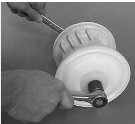
Step 12. Figure 12 Using two 1" sockets, remove diaphragm assembly from center section assembly.
